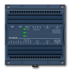
The **ECx-Light Series** Expansion Modules are microprocessor-based interfaces that extend the number of inputs and outputs provided by the ECLYPSE™ Connected System Controllers, ECLYPSE Connected VAV Controllers, ECL/ECB-PTU Series controllers, and ECL/ECB-VAV controllers. When connected to one of these HVAC programmable controllers, each ECx-Light-4 expansion module can control 4 ON/OFF lighting load and each ECx-Light-4D expansion module can control 4 ON/OFF or 1-10 V dimming lighting loads.
